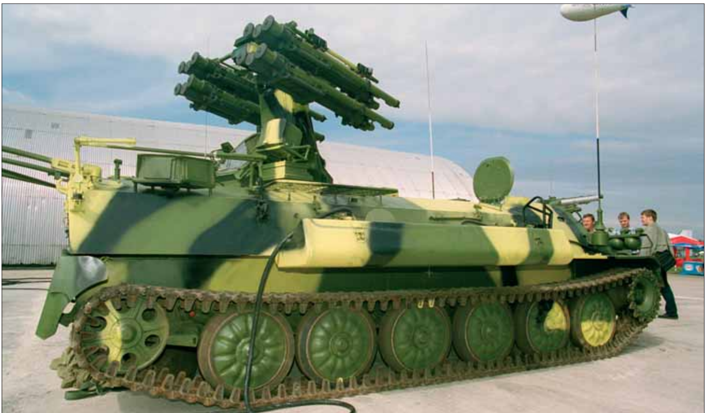
The Strelets SAM launch units can be fitted on any type of chassis and stationary mounts
